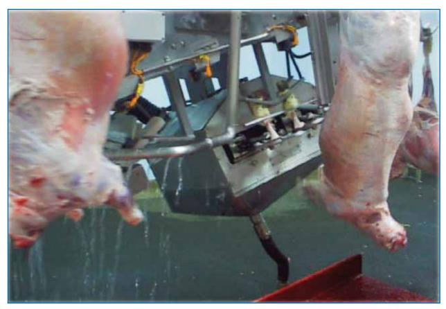
The Jarvis Model AHC2 - hydraulically operated hock cutter for sheep.
