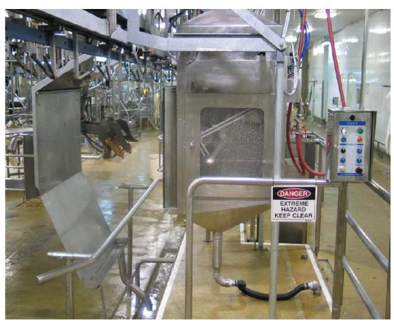
The Jarvis Model ABS-1 - hydraulic operated automatic brisket saw for sheep.
